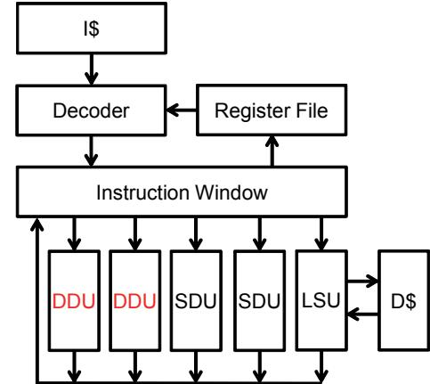
Fig. 2. Processor Core with Power Heterogeneous Functional Units
