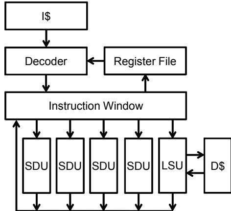
Fig. 1. Superscalar Processor Core
